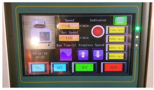
Select run time (1-1000 seconds), select speed (touch screen default speed 150r/min, 300r/min, 600r/min, 800r/min), also can choose stepless (press the down arrow) according to user needs, when selecting stepless shall be at standstill, and then select reversible press run key to operate. As follows (time setting)
